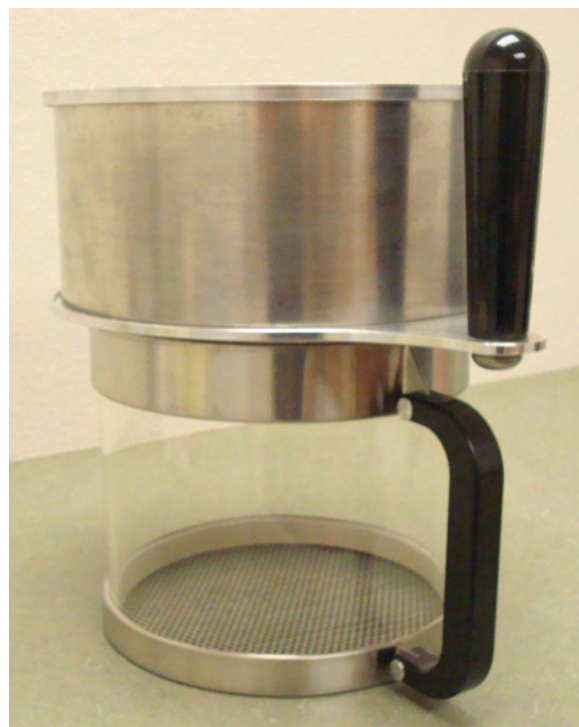
Completed roast chamber/chaff collector assembly.
