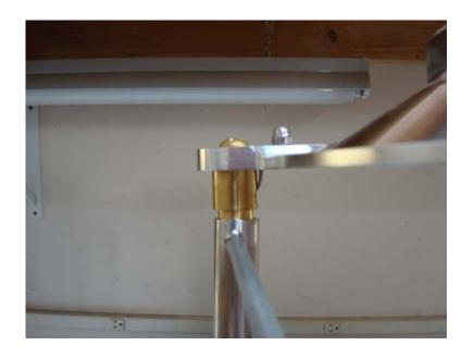
Reinstall the smoke box screws in reverse order, ensure that the washers are installed and the acorn nuts are tight.
