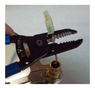
Cut old connectors from RTD, this will allow the RTD to be removed from the spacer.
