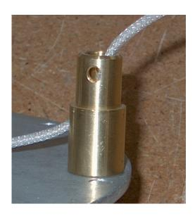
Ensure that the braided sleeve is passed through the spacer.
