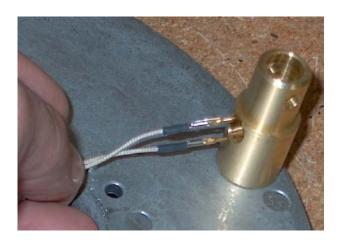
Insert RTD wires into the spacer hole and feed through. Ensure that the pins are not damaged in the process.
