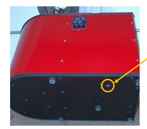
Tilt roaster on its side to access the valve adjustment screw.
