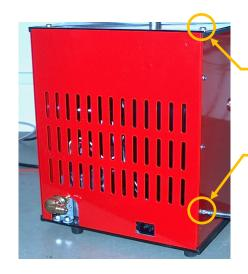
Loosen the 2 brass screws at the rear of the top panel a couple of turns to allow the back panel to be removed.
