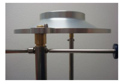
Remove smoke box screws using a #2 Phillips screwdriver and a 5/16" nut
