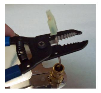
Insert RTD wires into the spacer hole and feed through. Ensure that the pins are not damaged in the process.
