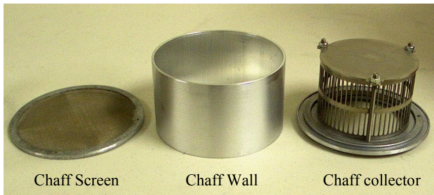
Chaff Collector Assembly
